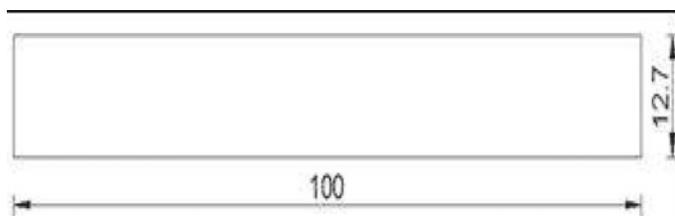
**Fig. 4** Flexural test specimen-part diagram
