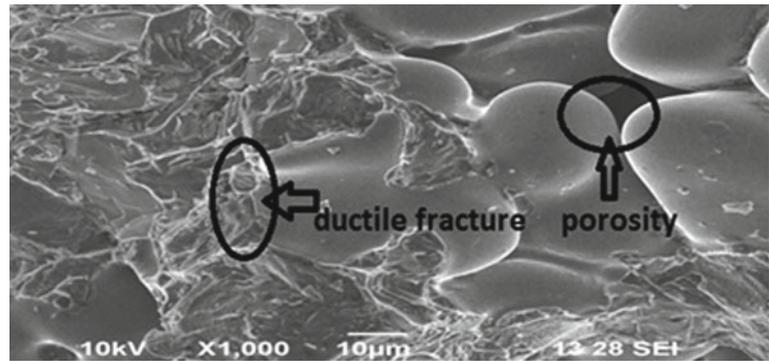
**Fig. 9** Fracture Surface of SEM Images with Nanoparticles
