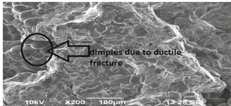
interacts with the atoms in the sample, it generates signals that can be detected and provide valuable information about the surface's topography and composition.
