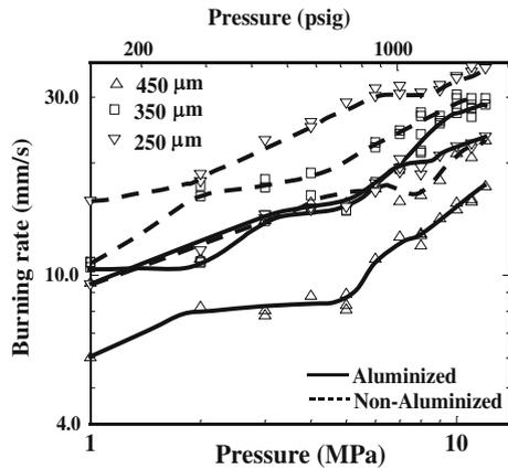
**Fig. 4** Effect of coarse AP size on the burning rates on TDI-cured propellants with a fine AP/binder ratio of 60/40, m size.  $\mu$  the fine AP size being 75  $\mu\text{m}$ , containing 15% Al of 15
