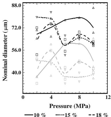
**Fig. 9** Effect of aluminum size on the agglomerate sizes of IPDI-cured propellants with a fine AP/binder ratio of 60/40, containing 15% Al, with the coarse and fine AP sizes being 450  $\mu\text{m}$  and 20  $\mu\text{m}$  respectively. (Grey–AMD and Black–SMD)
