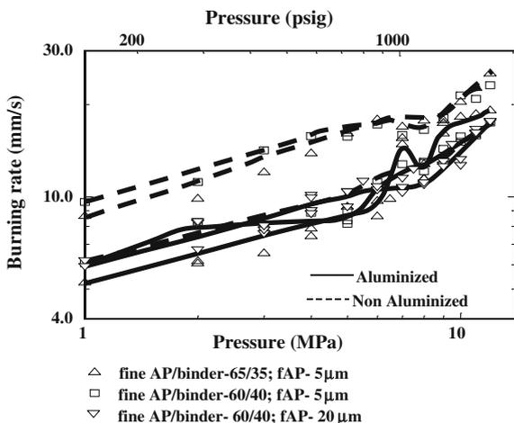
**Fig. 6** Effect of fine AP/binder ratio and fine AP size on the burning rates for IPDI-cured propellants with 450  $\mu\text{m}$  coarse AP along with the non-aluminized burning rates (Aluminized propellant-15% of 15  $\mu\text{m}$ .)
