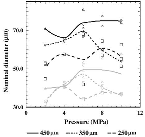
**Fig. 11** Effect of higher size fine AP size on the agglomerate sizes for TDI-cured propellants, containing 15% of Al with 15 μm size (SMD – dotted line ; AMD – solid line)
