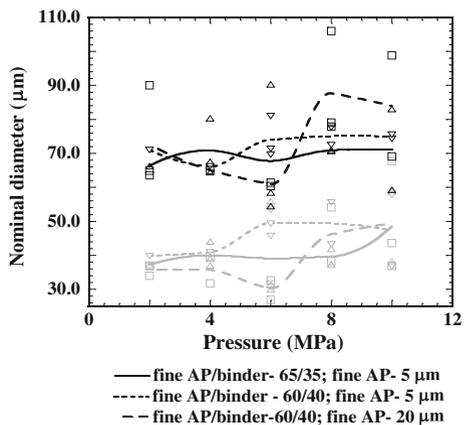
**Fig. 13** Effect of fine AP/binder ratio and fine AP size on the agglomerate sizes for IPDI-cured propellants with 450  $\mu\text{m}$  coarse AP containing 15% of Al with 15  $\mu\text{m}$  size (Grey-AMD and Black-SMD)
