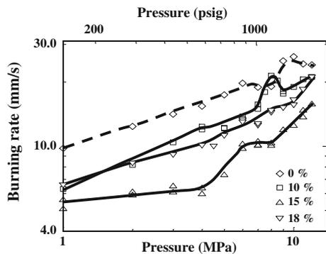
**Fig. 2** Effect of aluminum size on the burning rates of IPDI-cured propellants with a fine AP/binder ratio of 60/40, containing 15% Al, with the coarse and fine AP sizes being 450  $\mu\text{m}$  and 20  $\mu\text{m}$  respectively
