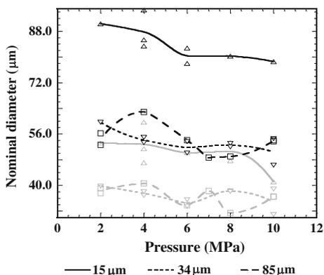
**Fig. 10** Effect of coarse AP size on the burning rates on TDI-cured propellants with a fine AP/binder ratio of 60/40, m size. (Grey—AMD and □ the fine AP size being 5 μm, containing 15% Al of 15 Black—SMD)
