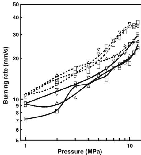
**Fig. 5** Effect of fine AP/binder ratio and fine AP size on the burning rates for TDI-cured propellants with 450  $\mu\text{m}$  coarse AP along with the non-aluminized burning rates
