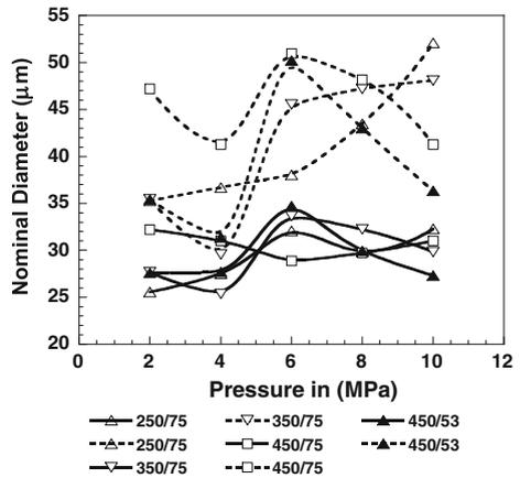
**Fig. 12** Effect of fine AP/binder ratio and fine AP size on the agglomerate sizes for TDI-cured propellants with 450 μm coarse AP, containing 15% of Al with 15 μm size (Grey—AMD and Black—SMD)
